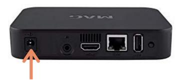
Remove the power cable for few seconds and then plug it back.
